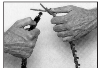
Pull belt end through two links.
