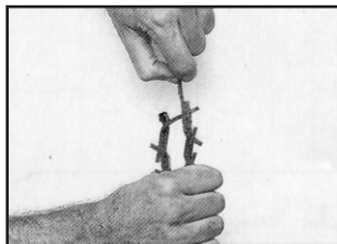
Pull end of link over tab.
